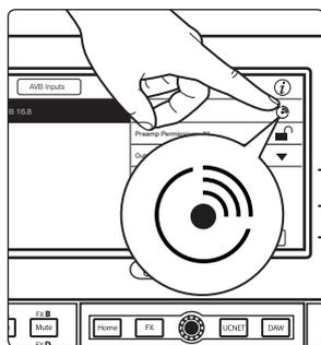
**Power User Tip:** In applications where you are using multiple NSB-series stage boxes of the same model, you can press the Identify button. This will flash the Power Network LED on the front of the selected NSB stage box from green to red, allowing you to quickly locate your selection.
