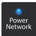
**Power Network.** This LED displays power and network connectivity. When the LED is red, no network is available. When it is blue, the NSB stage box is connected to an AVB network.
